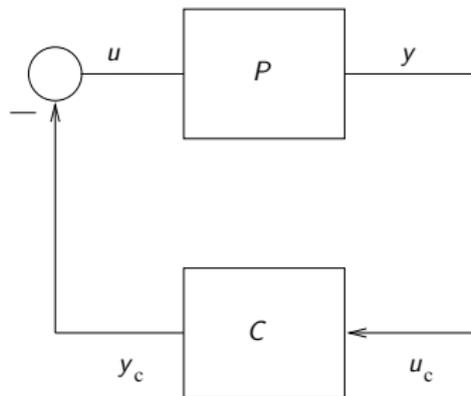
By **compositionality**, the closed-loop system is the pH system
