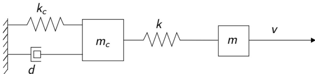
Figure: Plant mass and controller mass-spring-damper system
