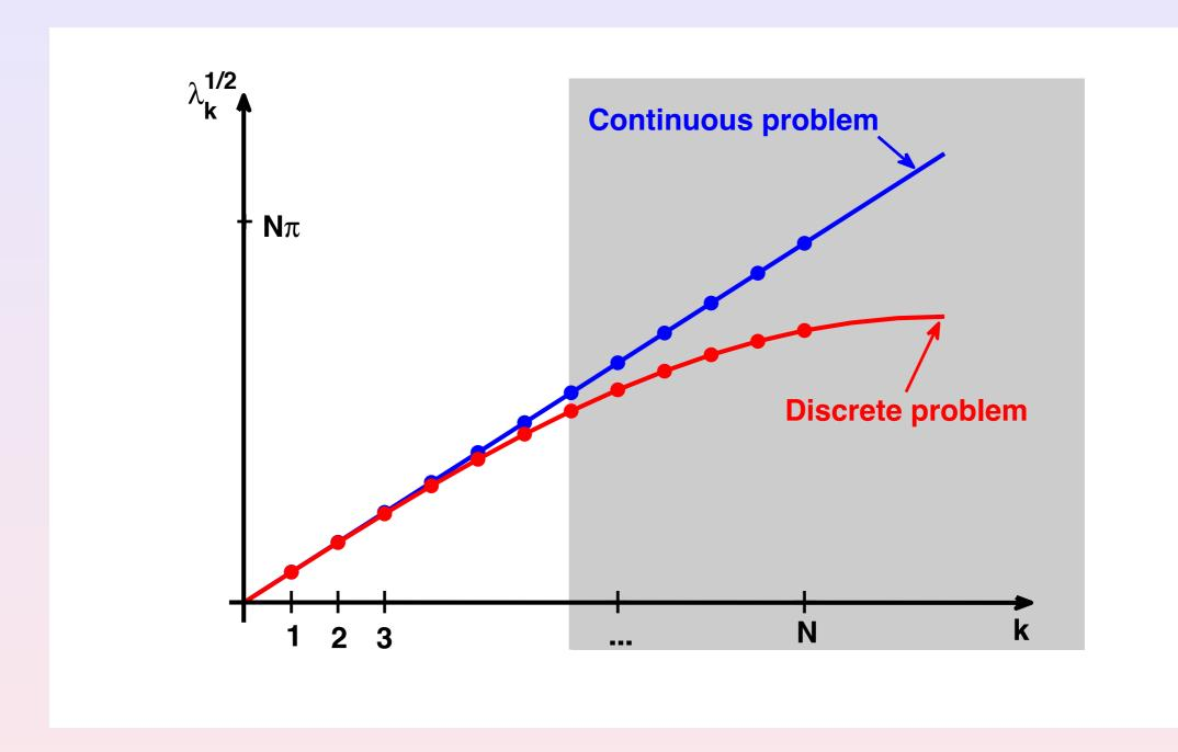
To filter the high frequencies, keeping the components  $k \leq \delta/h$  with  $0 < \delta < 1$ . Then the group velocity remains uniformly bounded below and uniform observation holds in time  $T(\delta) > 2$  such that  $T(\delta) \to 0$
