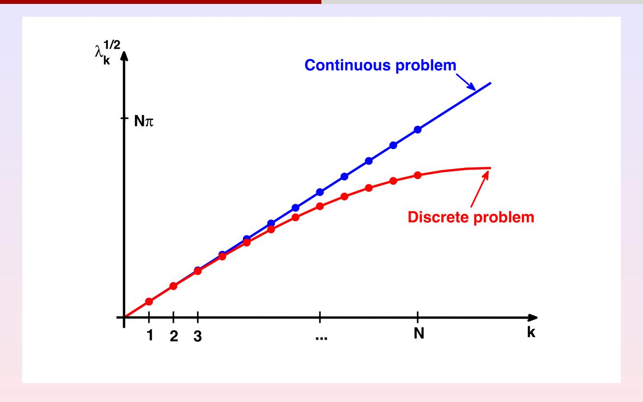
Graph of the square roots of the eigenvalues both in the continuous and in the discrete case. The gap is clearly independent of k in the conflex case while it is of the order of h for large k in the discrete one.
