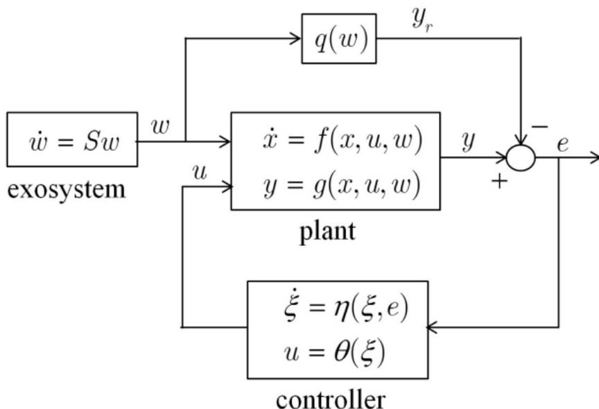
This diagram shows the closed-loop system of the plant and the controller, driven by the exosystem  $S$ . The problem is to ensure that the closed loop system with  $w = 0$  is locally exponentially stable and for small enough initial states,  $e(t) \rightarrow 0$ .
